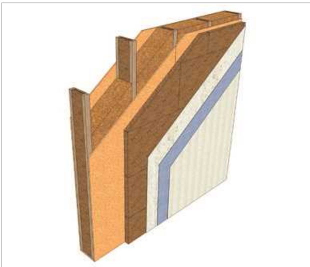
Timber frame with external board material
